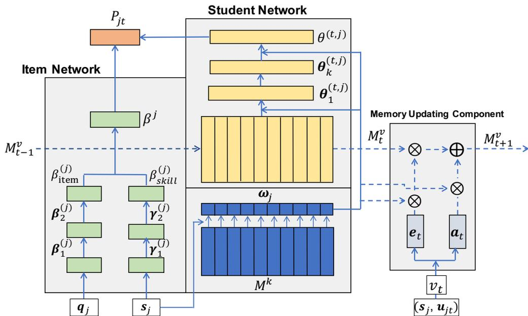
Figure 4: Network architecture of the proposed method with independent student and item networks for KT. The yellow components are associated with the student network. The green components are associated with the item network. In addition, the right side of figure presents the memory updating component. The designations  $\otimes$  and  $\oplus$  respectively represent element-wise multiplication and addition.
