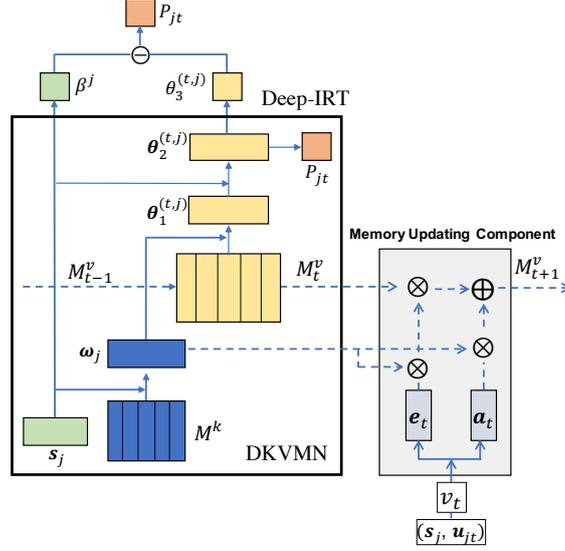
Figure 1: Network architecture of DKVMN and Deep-IRT. The underside of the structure describes DKVMN; the whole structure describes Deep-IRT. The blue components represent the process of getting the attention weight. The yellow components are associated with the student network and the process of updating the value memory. The green components are associated with the item network. The designation  $\ominus$  represents subtraction.
