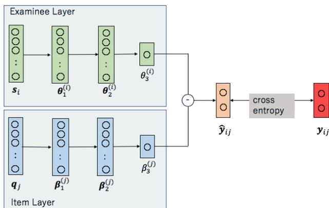
Figure 2: Network architecture of the proposed method with independent student and item networks for test theory. The green components are associated with the student network. The blue components are associated with the item network. The designations  $\odot$  represents element-wise multiplication and subtraction.
