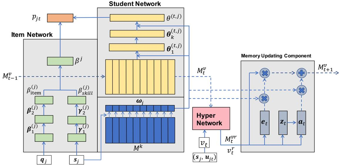
Figure 5: Memory updating component of the proposed method with hypernetwork. The proposed hypernetwork is located at the beginning of the Memory Updating Component. It estimates the optimal forgetting parameters by balancing both the current input data and the past latent variable before the model updates the latent variable.
